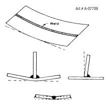
Figure 4-33: Examples of Distortion
