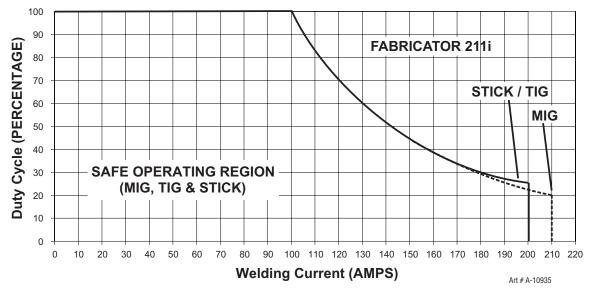
Figure 2-2: Fabricator 211i Duty Cycle on 230VAC
