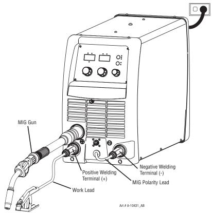
Figure 3-14: Setup for MIG Welding with Gasless MIG Wire
