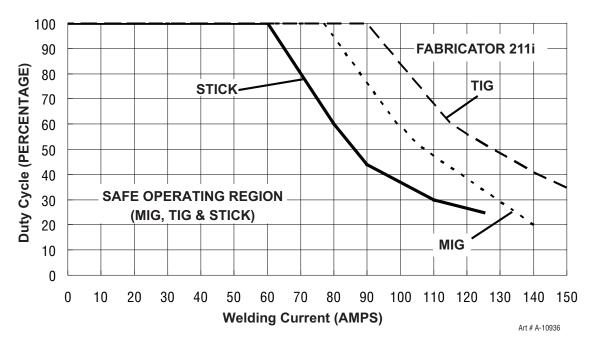
Figure 2-3: Fabricator 211i Duty Cycle on 110VAC
