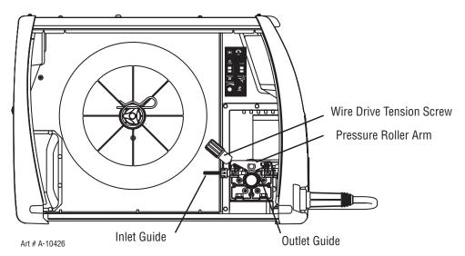
Figure 3-8: Wire Drive Assembly Components
