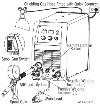
Figure 3-15: Setup for Spool Gun Welding with Gas Shielded MIG Wire
