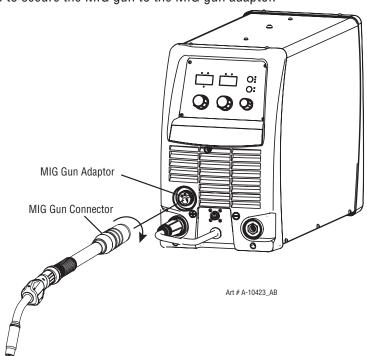
Figure 3-5: Attaching MIG Gun
