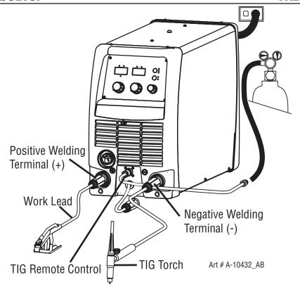
Figure 3-16: Setup for TIG Welding
