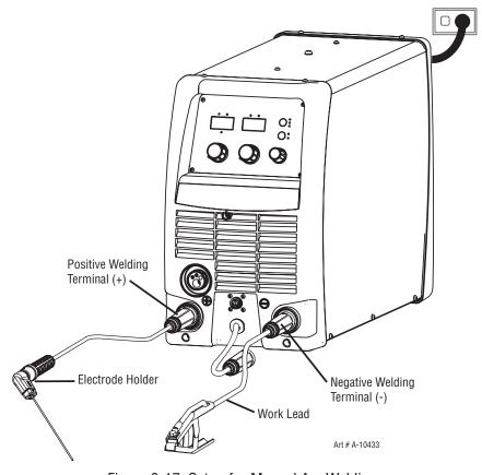
Figure 3-17: Setup for Manual Arc Welding.
