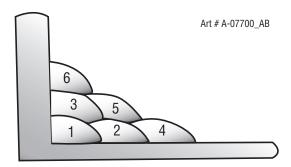
Figure 4-24: Multi-runs in HV Fillet Weld
