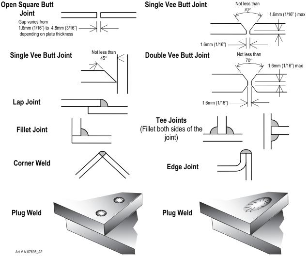
Figure 4-19: Typical Joint Designs for Arc Welding
