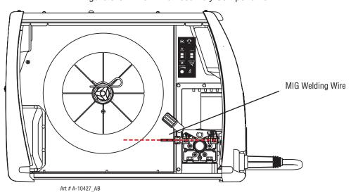
Figure 3-9: MIG Welding Wire - Installation
