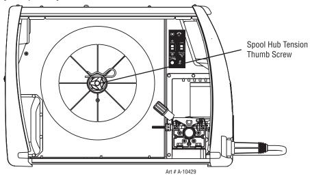
Figure 3-12: Wire Reel Brake
