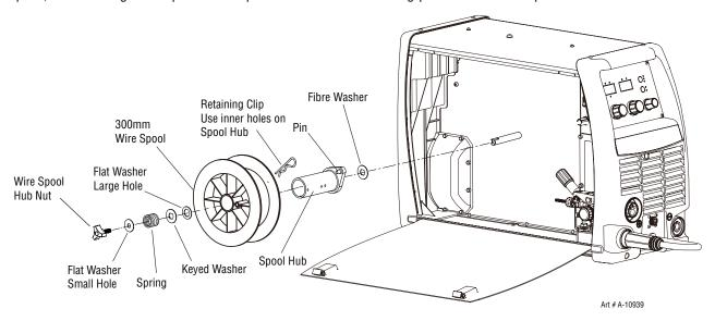
Figure 3-6: 300mm 15kg Spool Installation
