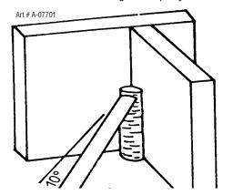
Figure 4-25: Single Run Vertical Fillet Weld
