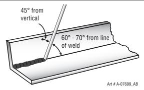
Figure 4-23: Electrode Position for HV Fillet Weld
