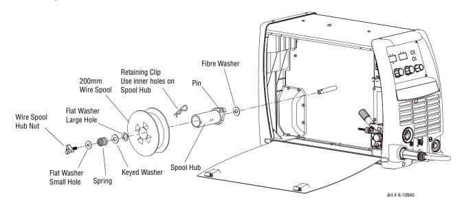
Figure 3-7: 200mm 5kg Spool Installation
