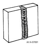
Figure 4-15: Vertical Position, Butt Weld
