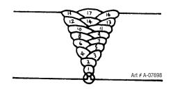
Figure 4-22: Weld Build up Sequence
