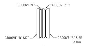
Figure 3-10: Dual Groove Feed Roller
