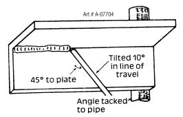
Figure 4-28: Overhead Fillet Weld
