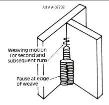
Figure 4-26: Multi Run Vertical Fillet Weld
