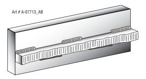
Figure 4-37: Staggered Intermittent Welding
