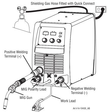
Figure 3-13: Setup for MIG Welding with Gas Shielded MIG Wire
