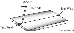
Figure 4-21: Butt Weld
