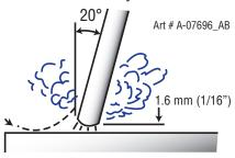
Figure 4-20: Striking an Arc
