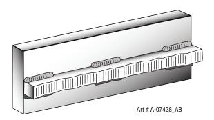
Figure 4-36: Chain Intermittent Welding
